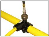
**14** Remove cap, then insert drive key (use drive key 33-5505-00) into punch.
